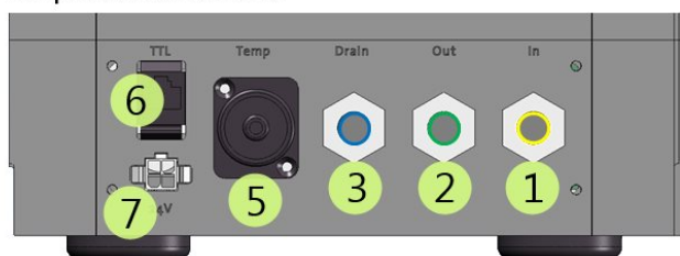
Figure 16 The back panels of the DanioVision Observation Chamber (top) and the Temperature Control Unit (bottom). The numbers of the connectors / ports are also described in the text above.
