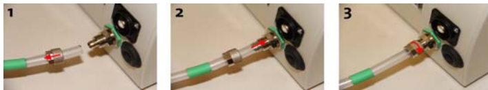
Figure 15 How to connect a tube to a TCU connector. 1 - Slide the nut of the connector onto the tube, 2 - Connect the tube to the connector, 3 - Screw the nut onto the connector.
