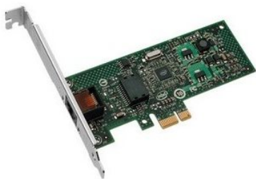
Figure 8 An Ethernet card for connecting the DanioVision camera to the EthoVision XT computer.
